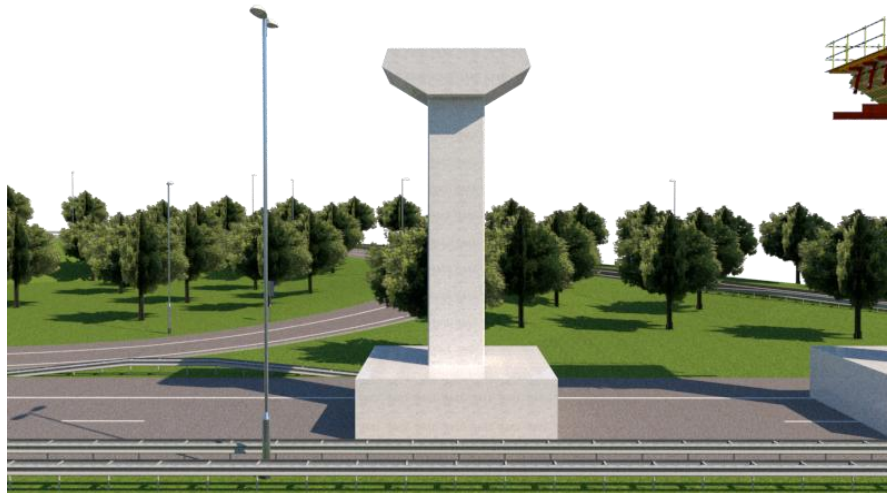
Gambar 1. 3D Pier Head
