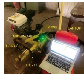
Gambar 4.1 Instalasi Dynamometer rem cakram
